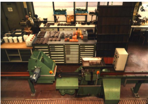
Photo 1: Concrete roof tile machine (extrusion press), Schade (1970)
