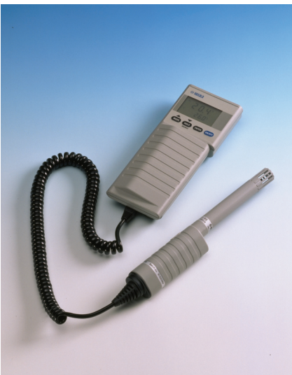
HMI41 with the HMP45 probe.
