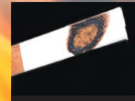
When fire is extinguished, simply scrape away the char barrier and damage is minimized
