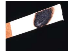
Char barrier reflects heat and protects the underlying substrate
