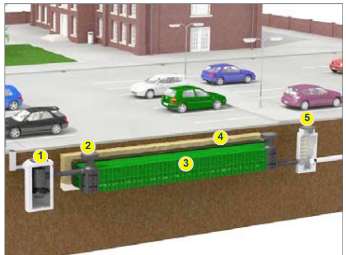
Figure 1: Components of a Stormbloc™ storage or infiltration system
