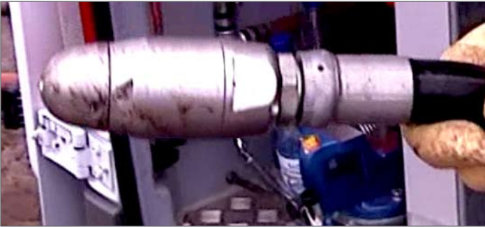
Figure 8: A rotating pressure nozzle attachment for pressure jetting
