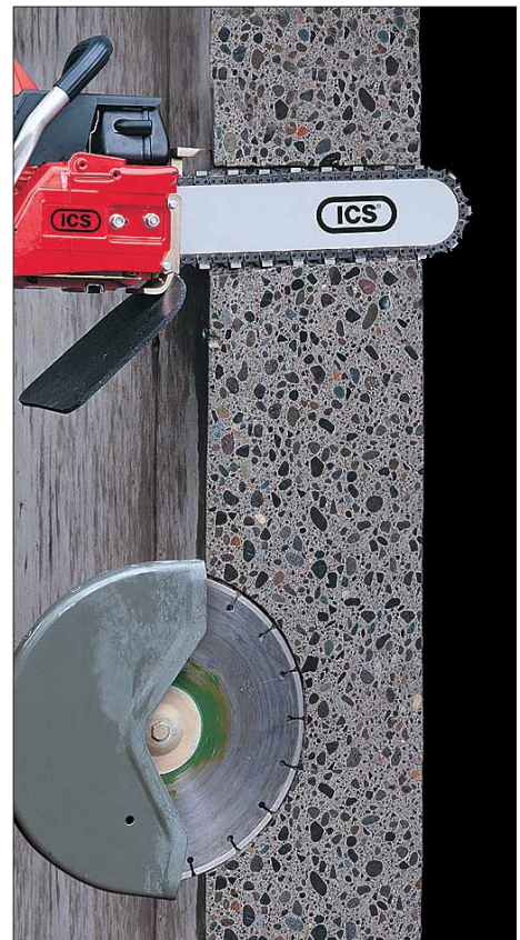
ICS concrete cutting chainsaw vs. diamond blade
