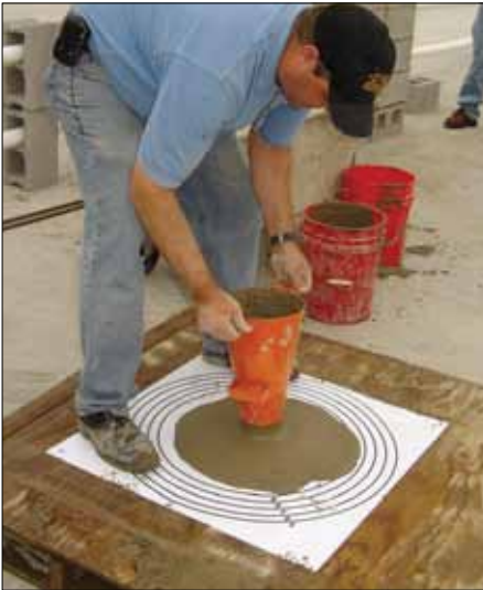
SCG Slump-Flow test targets a 20" (508 mm) spread in 2 - 5 seconds.
